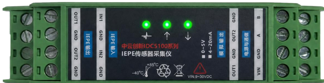
Figure 5-1 Interface and Indicator Locations
